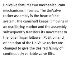
UniValve can also completely deactivate individual valves, fully shutting down their respective cylinders. Now, that's downsizing on demand.
