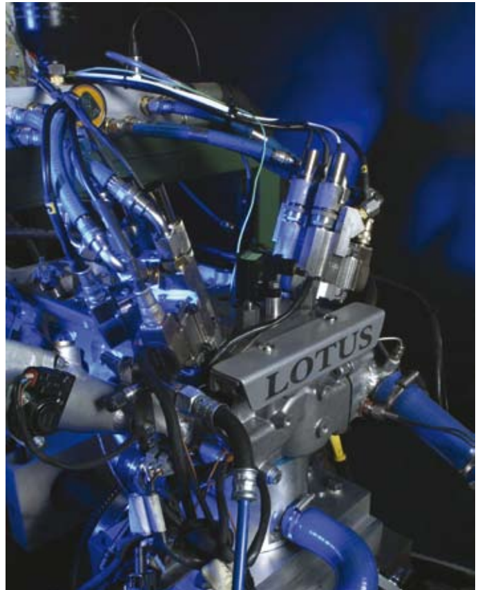
The Lotus AVT research engine uses conventional closing springs for valves
