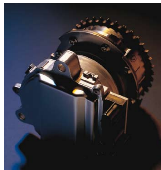
The motor driven electric variable valve from Denso in Japan makes use of an electric motor in the actuator mounted axially with inlet camshafts that spins faster than the shaft in order to advance the timing. Debuting in the Lexus LS460 earlier this year, Denso's system realizes better response at low engine speeds and temperature levels
